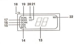
LCD Numerical Channel Display - Indicates Channel Number in use. Weather Channels are displayed as single digits. (Example: 0, 1, 2, 3, etc.) Communication Channels are displayed as two digits (Example: 01, 02, 03, etc.).
